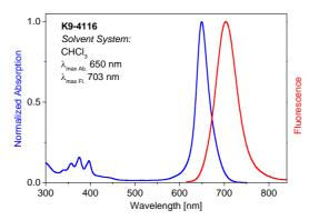
Absorption and emission spectrum of **K9-4116** in chloroform
